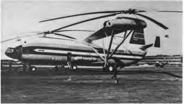
Figure 6-56. Mi-12 HOMER. HOMER is the largest helicopter in the world. It is easily recognized by the two large wing-tip rotors, and is shown here in use by AEROFLOT, the Soviet civilian airline.
